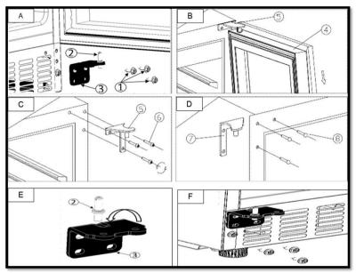
1 Screws 2 Hinge axis 3 Lower hinge 4 Door 5 Top hinge (Right) 6 Screws 7 Top hinge (Left) 8 decorative nail
